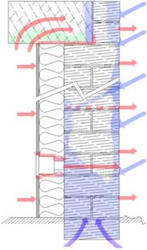
*Solid internal insulation with vapour impermeable barrier or insulation. E2*
