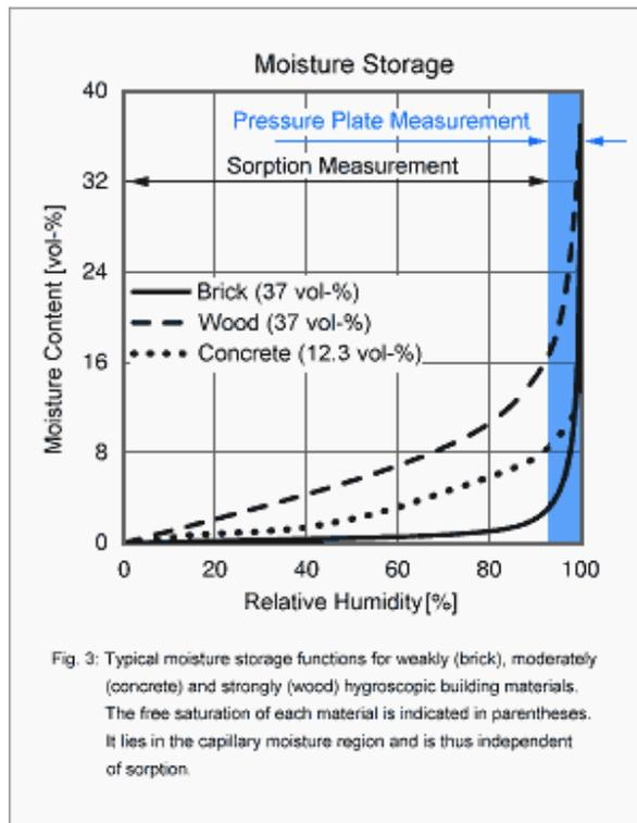
In this chart the blue area at over 95% RH indicates the effect of water transported by capillary condensation. This in itself is also different from capillary transport of water as a liquid, which occurs in different sized pores and is a different mechanism altogether (see footnote 13). The hygroscopic capacity (measured as the change in equilibrium moisture content at different humidities) is here shown to operate only up to around 90 - 95% depending on the materials.<sup>9</sup>
