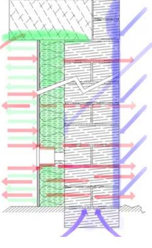
*Solid internal insulation with vapour open hygroscopic insulation.*
