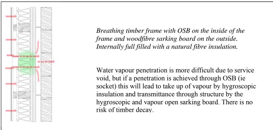
It is a simple step to put the OSB on the inside and then put a vapour open board or membrane on the outside, which is indeed what TRADA suggested 20 years ago and which is common practice abroad. The advantage of an insulating woodfibre board is that it is both warm, thus preventing
