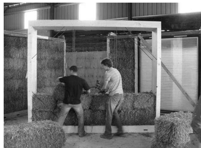
Figure 2. Panel construction process in ‘flying factory’
